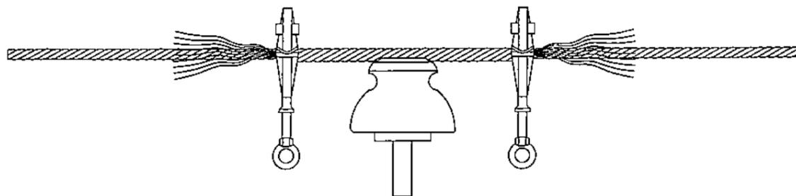
FOR TOOL APPLICATION, INSERT HALF OF THE REINFORCEMENTS IN ONE CAVITY AND ENTER THE OTHER HALF IN THE OTHER CAVITY OF THE OPEN WRENCHES, KEEPING THE ENDS EVEN. HOOK WRENCHES OVER THE CONDUCTOR AND CLOSE JAWS. SPACE WRENCHES APPROXIMATELY ONE REINFORCEMENT PITCH APART AND TWIST THEM IN THE SAME DIRECTION AS THE LAY OF THE CONDUCTOR. WIND EACH WRENCH TO THE END OF THE REINFORCEMENT AND REMOVE.
