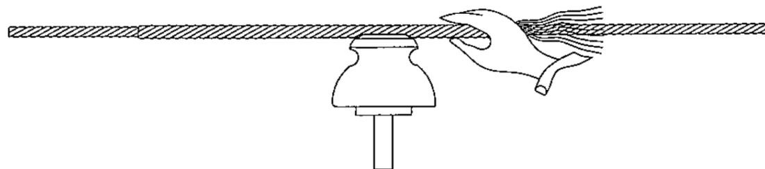
FOR HAND APPLICATION, HOLD ONE OR MORE REINFORCEMENTS AGAINST THE CONDUCTOR WITH MIDPOINT AT THE INSULATOR, AND ROTATE IN SAME DIRECTION AS THE LAY OF THE CONDUCTOR, FOR THREE OR FOUR INCHES EACH SIDE OF CENTER. IN LIKE MANNER APPLY REMAINING REINFORCEMENTS TO CENTER SECTION. AFTER ALL HAVE BEEN STARTED, COMPLETE THE APPLICATION BY A ROTARY OUTWARD WIPING MOTION OF THE HAND. MAKE CERTAIN THAT THE ENDS SNAP INTO PLACE IN PROPER ORDER.
